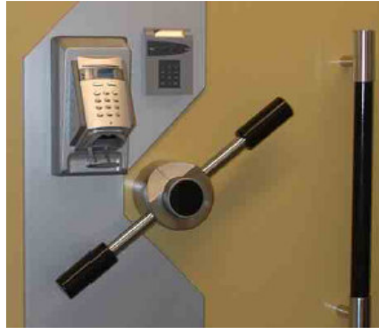
Figure 8: Vein scan access to bank safe
